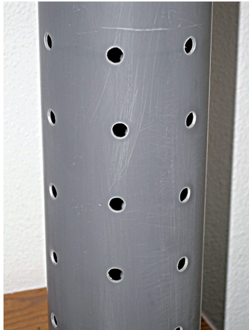
Fig. 11. Detail of holes drilled along middle part of component A of a MSS trap (© MNCN; photographer: M.A. Alonso-Zarazaga).
