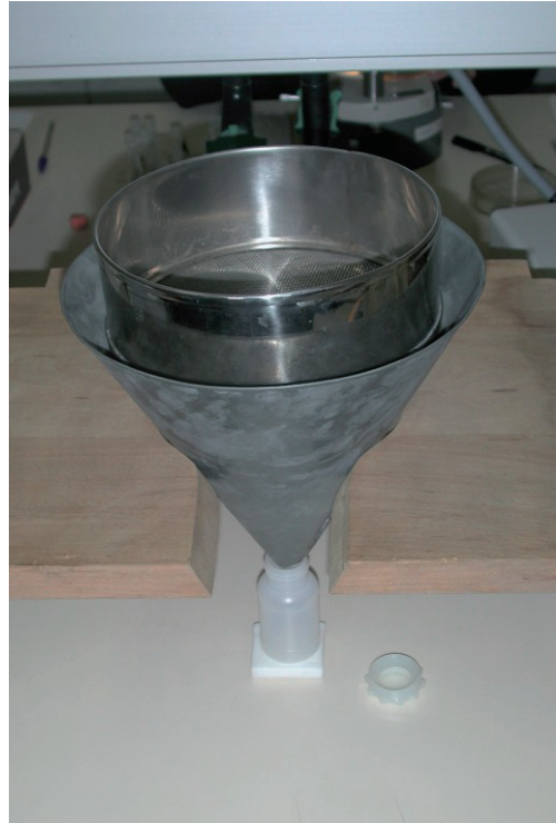
Fig. 14. Berlese collector formed by a sieve, a funnel, a holder and a plastic container with preservative. Leaded gauze is not shown. (© MNCN; photographer: Teresa Domingo-Quero).
