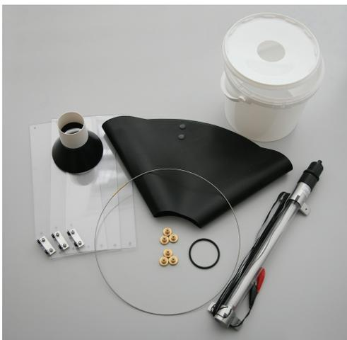
**Fig. 8.** The same trap, disassembled. Top right: container. Right: actinic tube inside a Plexiglas cover with cable. The electronics are housed in the black top cap. Left: Plexiglas baffles and lower part of funnel. Centre: collapsible funnel with stabilising ring, screws for fastening baffles to tube housing, rubber ring for fastening lower part of funnel to container lid. (Photo by A. Steiner).
