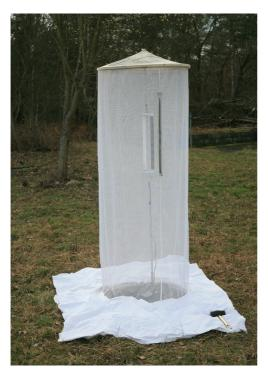
**Fig. 4.** Personal light-trapping. Two battery-powered 15 W fluorescent tubes in a gauze cylinder ("tower"). (Photo by A. Steiner).
