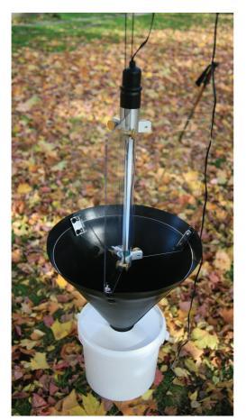
Fig. 7. A hanging light-trap without raincover, showing three baffles around a 6 W actinic tube, a collapsible funnel made of thick plastic film, and a bucket as container. (Photo by A. Steiner).
