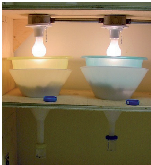
Fig. 7. Berlese-Tullgren funnels. (Photo by Heather Proctor).
