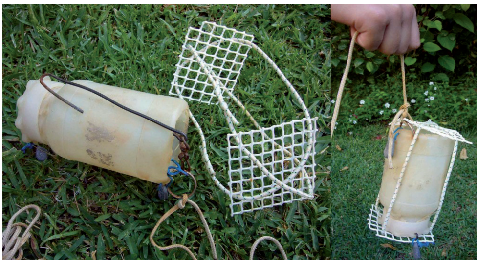
Fig. 13. A simple trap to sample stygofauna in cave lakes and pools. The plastic grid frames can be added to protect the animals eventually attracted by bait from crabs, eels or other potential predators. (Photo by Damia Jaume).
