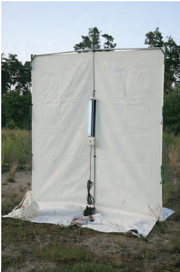
Fig. 1. Personal light-trapping. The sheet method. A white linen sheet mounted on a frame of aluminium poles, with two battery-powered 15 W fluorescent tubes, one actinic, one black.(Photo by A. Steiner).
