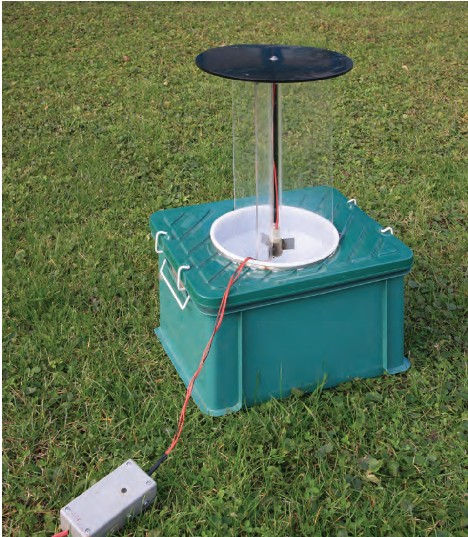
Fig. 9. A ground light-trap with a rain cover and three baffles around an 8 W black-light tube. The container is a commercially available plastic box. The black dot on the small grey box containing the electronics is the photoelectric cell. (Photo by A. Steiner).
