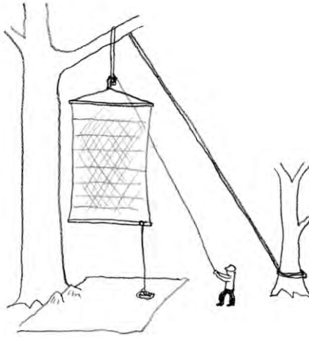
Fig. 5. Schematic view of a vertical canopy mist net (modified after Kunz et al. , 1988). The net is hoisted via a pulley into the canopy. A tarp is put on the floor on which the mist net can be lowered when bats are extracted from the net.
