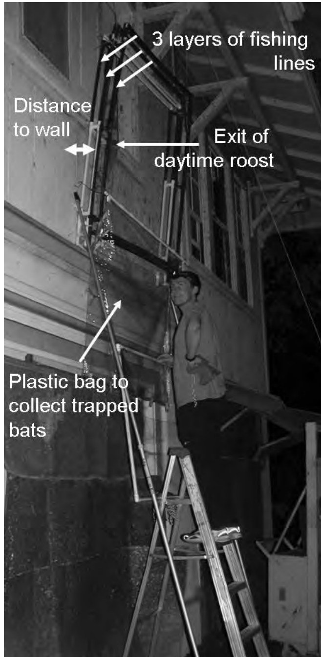
Fig. 6. Harp trap set up in front of the exit hole of a daytime roost. Two bat species, Noctilio albiventris and Molossus molossus emerged from the roost, hit the layer of fishing lines and tumbled into the plastic bag from which they were quickly recovered and transferred to linen bag. (Photo by D.K.N. Dechmann).
