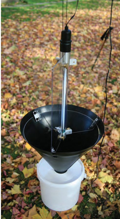
Fig. 7. A hanging light-trap without rain-cover, showing three baffles around a 6 W actinic tube, a collapsible funnel made of thick plastic film, and a bucket as container. (Photo by A. Steiner).
