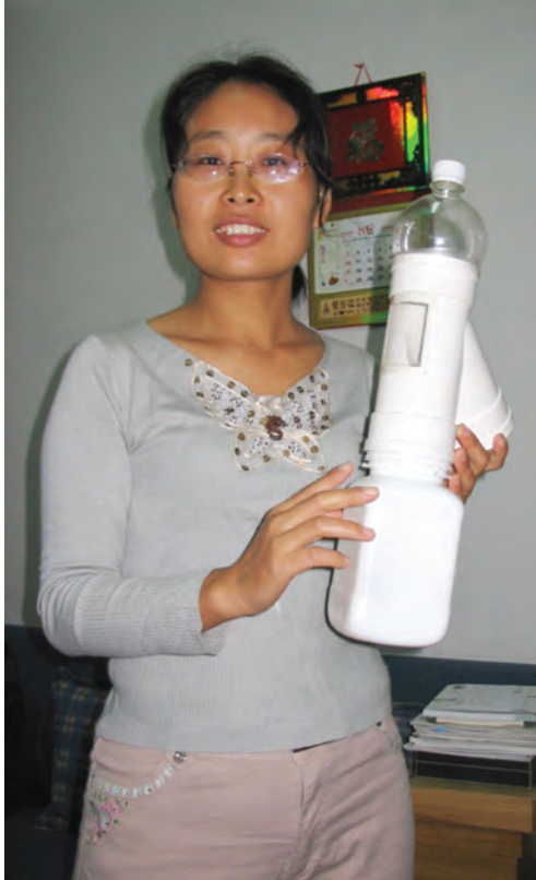
Fig. 7. White UPVC collector for Malaise trap (Hangzhou type) (75 mm/45 degrees, 3.2 mm + insert) with 1 l bottle. (Photo by C. van Achterberg).
