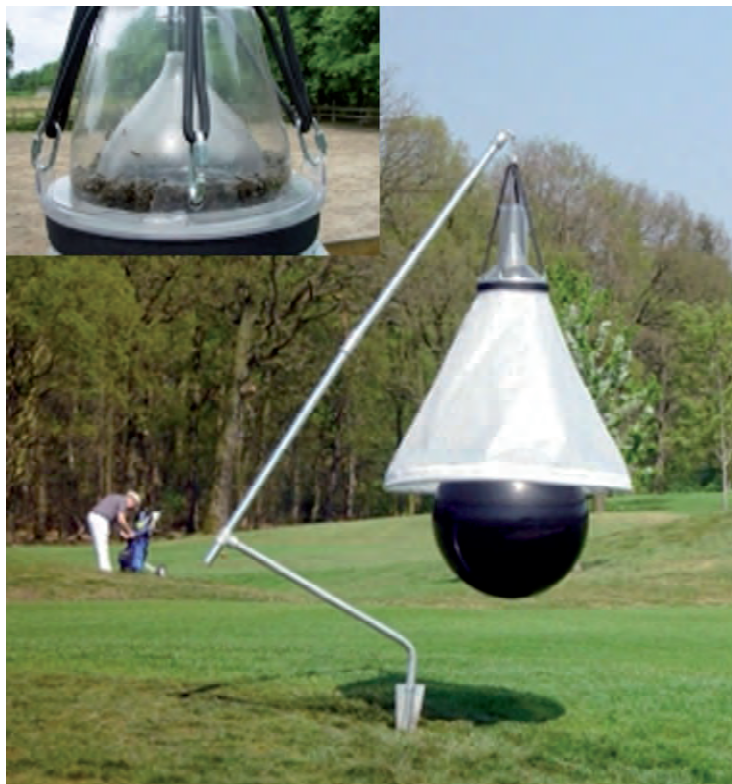
Fig. 22. Ball and hood (LOER-2007) trap for collecting horse flies. Left collector with dead flies (From: www.dazenval.nl ).
