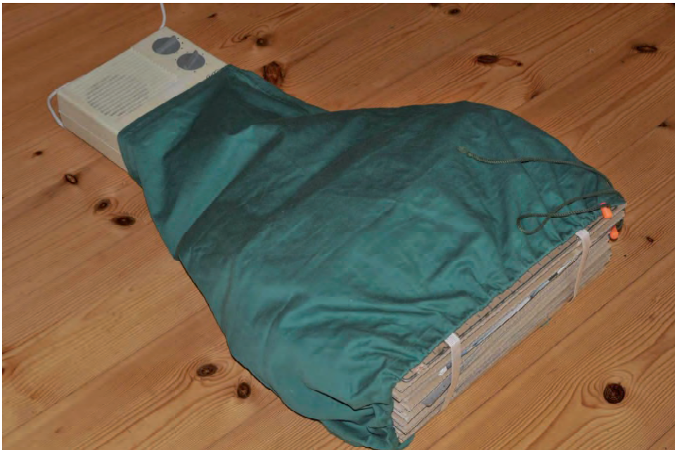
Fig. 4. Drying set with an electric heater and a funnel of fire resistant canvas.
