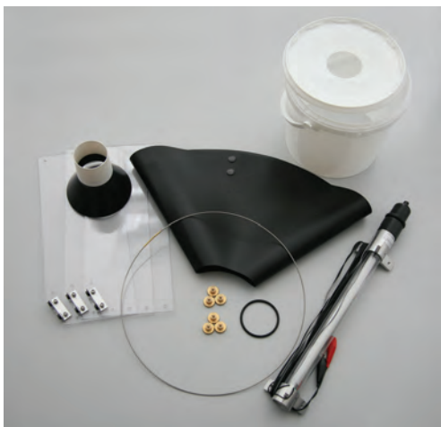
Fig. 8. The same trap, disassembled. Top right: container. Right: actinic tube inside a Plexiglas cover with cable. The electronics are housed in the black top cap. Left: Plexiglas baffles and lower part of funnel. Centre: collapsible funnel with stabilising ring, screws for fastening baffles to tube housing, rubber ring for fastening lower part of funnel to container lid. (Photo by A. Steiner).
