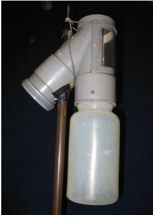
Fig. 5. Large grey PVC collector for Malaise trap (75 mm/45 degrees, 3.2 mm + insert) with 1 l bottle. (Photo by C. van Achterberg).
