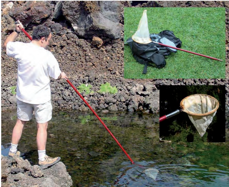
Fig. 12. Small plankton net screwed to an extensible handle. The folded handle and unscrewed net can be carried out with ease along the narrow cave passages, and assembled to reach even the deeper parts of the pools and cracks from the shore (Photo by Damia Jaume).
