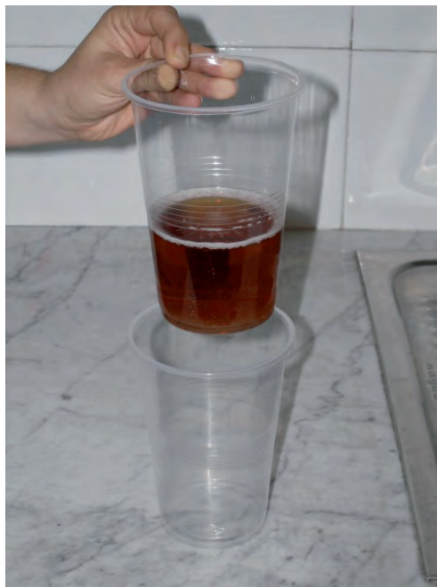
Fig. 8. Placement of inner beaker cup container with killing-preserving liquid inside an outer similar container (© MNCN; photographer: M.A. Alonso-Zarazaga).
