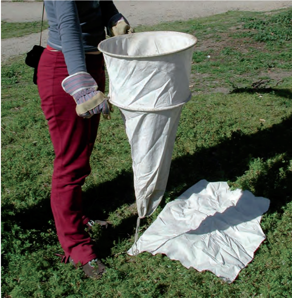
Fig. 3. Winkler-Wagner elector ready to be used in the field (© MNCN; photographer: Manuel Sánchez-Ruiz).
