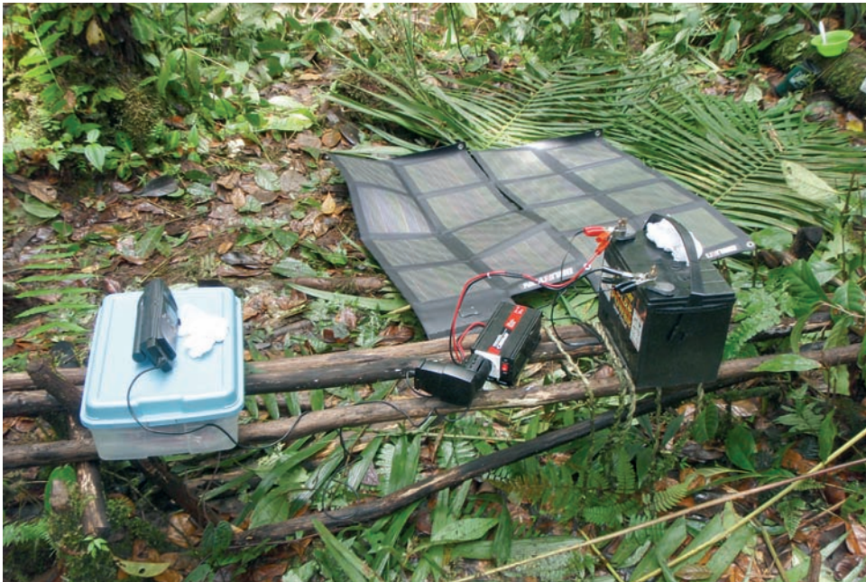
Fig. 20. Electric power provided by solar panels, here charging the emergency satellite phone. See text for details. (Photo by P. J. R. Kok).
